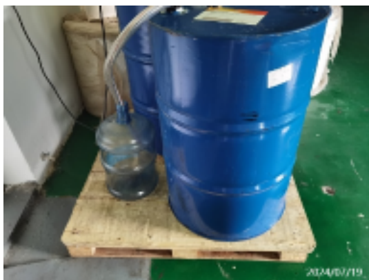
NC-No secondary containment.jpg
